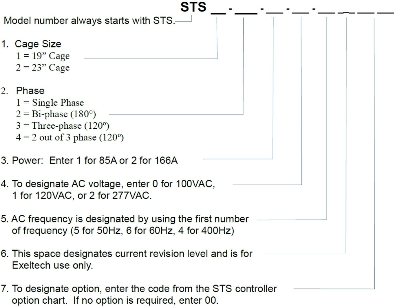
Example: 19" Three phase 20kW 120VAC 60Hz – STS1-3-2-1-6100
